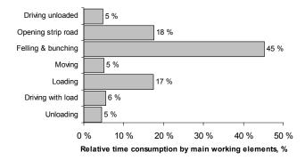
**Figure 3.** Main elements of the energy wood harwarders effective working time
