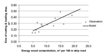
Figure 7. The size of cutting and loading stop as a function of the energy wood concentration
