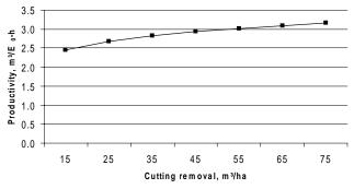
Figure 12. The effective hour productivity of energy wood logging with harwarder as a function of cutting removal. Tree volume of removal is 25 dm3 and forwarding distance 250 m
