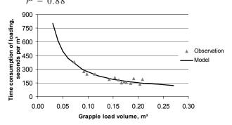
**Figure 5.** Time consumption of loading as a function of grapple load volume
