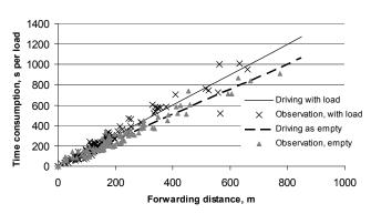
**Figure 8.** Time consumption when driving unloaded and with load as a function of forwarding distance
