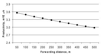
Figure 11. The effective hour productivity of energy wood logging with harwarder as a function of forwarding distance. Tree volume of removal is 25 dm<sup>3</sup> and accumulation of energy wood 50 m<sup>3</sup> per hectare
