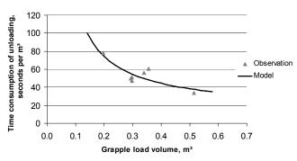
**Figure 9.** Time consumption of unloading as a function of grapple load volume
