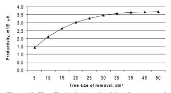
Figure 10. The effective hour productivity of energy wood logging with harwarder as a function of tree volume. Forwarding distance 250 m and accumulation of energy wood 50 m<sup>3</sup> per hectare
