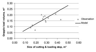
Figure 6. The grapple load volume according to size of cutting and loading stop
